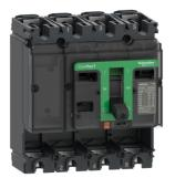
Circuit breaker basic frame, ComPacT NSX160F, 36kA/ 415VAC, 4 poles, 160A frame rating, without trip unit
